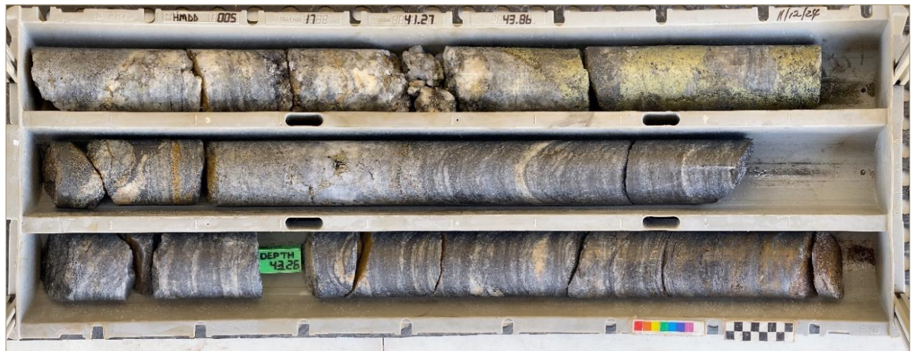
Photograph 3: PQ Core Packed and Marked in a PVC Core Box
