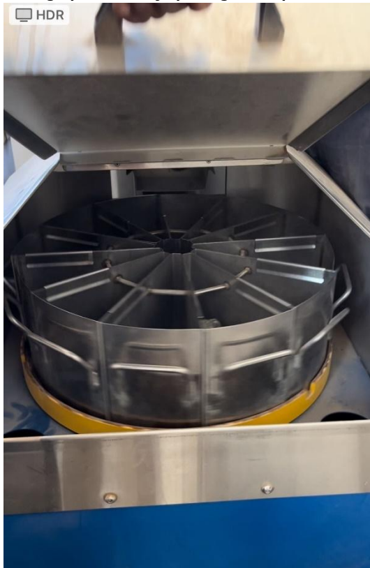
Photograph 14: Rotary Splitting of Samples
