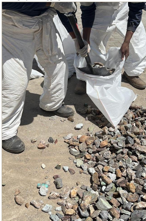
Photograph 9: Bagging of Crushed and Screened Coarse Fraction
