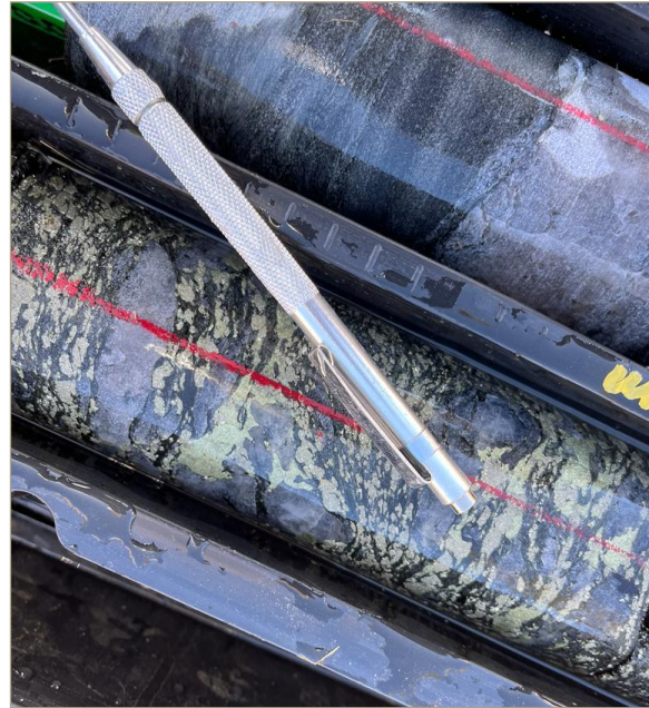
Figure 2 :Pyrite Mineralisation within Drill Core
